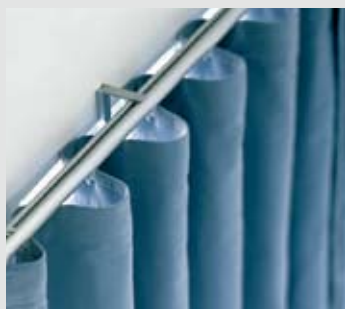
Example of largest Wave® curtain effect using 80mm glider-cord with 160mm curtain hook spacing.
